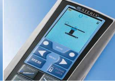
Easy-To-Read LCD Large fonts and intuitive graphics provide robust information on table position, service alerts, battery power and more.
