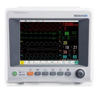
The Edan iM50 patient monitor with G2 Co2 allows the user to evaluate patient status at a glance of the screen and also includes optional End Tidal Co2 monitoring (sidestream). The 8.4", bright, color display is easily seen, even from a distance. The user friendly design and menus make the system easy to use and understand. This unit is designed with transportation in mind, and this compact, lightweight monitor can be easily taken anywhere.
