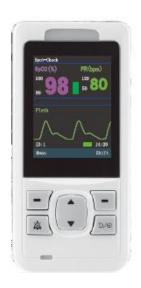
The Biolight M800 features a 2.4" LED display that is compact and light for carrying and handling. The M800 functions include: automatic display rotation, two selectable working modes, spot check and continuous monitoring.
