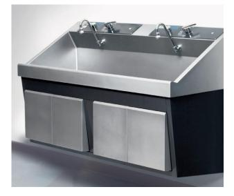
The Steris Amsco Flexmatic dual station scrub sink is a heavy duty, hospital grade surgical scrub sink that has two independent bays. The water flow is controlled by knee actuation. The operator simply presses their knee against the stainless steel kick plate to start the water flow. Stopping the water flow is as easy as simply pressing the kick plate again.
