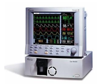
The Datascope Passport 2 anesthesia monitor allows the user to evaluate patient status at a glance of the screen. The large (10.4"), bright, color display is easily seen, even from a distance. The user friendly design and menus make the system easy to use and understand. For anesthesia use, the Gas Module is attached underneath the Passport 2 and interfaces to measure EtCo2, FiO2, O2, N20, and 5 anesthetic agents during procedures.
